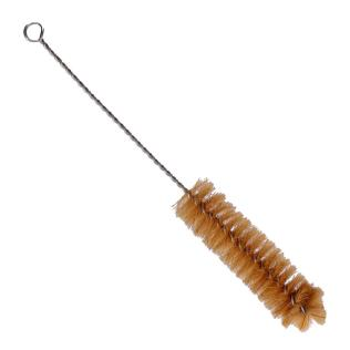
A tube brush in engineering testing laboratories is used for cleaning narrow, cylindrical surfaces such as
