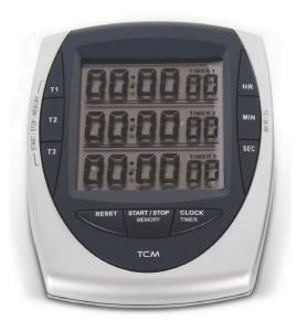
A stopwatch in engineering testing laboratories is used to measure time intervals accurately during various tests, such as setting time of cement, flow duration, or penetration tests. It ensures precise timing, which is crucial for reliable and repeatable test results.
