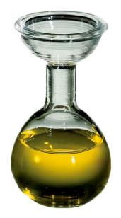
• A flask for a Saybolt viscometer in engineering testing laboratories is used to hold the sample liquid during viscosity testing. It is designed to fit the viscometer and ensure accurate measurements of the fluid's resistance to flow at a specific temperature, which is essential in evaluating the viscosity of oils and other liquids.
