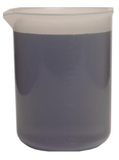
• A plastic beaker in engineering testing laboratories is used for holding, mixing, and heating liquids or chemicals. It is lightweight, durable, and resistant to breaking, making it ideal for everyday use in various laboratory procedures where glass beakers may be too fragile or impractical.
