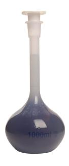
• A plastic volumetric flask in engineering testing laboratories is used for accurately preparing and diluting solutions to a precise volume. It is lightweight and durable, making it suitable for handling chemicals and liquids, especially when glass flasks are prone to breakage. It ensures precision in chemical analysis and sample preparation.
