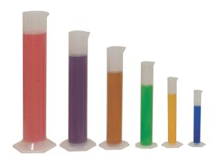
• A plastic measuring cylinder in engineering testing laboratories is used for accurately measuring the volume of liquids. It is lightweight and durable, making it suitable for handling a variety of chemicals or materials, especially when glass containers might be too fragile or heavy. It provides precise measurements for experiments and sample preparation.
