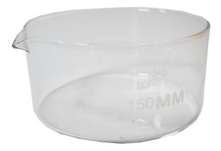
• A crystallizing dish in engineering testing laboratories is used for evaporating solvents and facilitating the crystallization of dissolved substances. Typically made of glass or porcelain, it allows for the gradual formation of crystals, often used in chemical analyses and purification processes.
