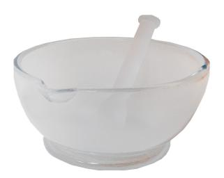
• A glass mortar and pestle in engineering testing laboratories are used for grinding and mixing materials, particularly for substances that may react with porcelain or other materials. The smooth surface of glass ensures no contamination and is ideal for preparing fine powders or combining chemicals in precise quantities for testing.
