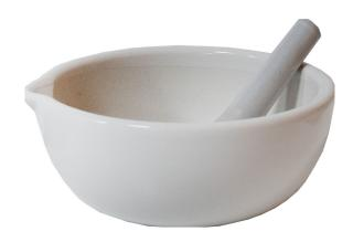
A porcelain mortar and pestle in engineering testing laboratories are used for grinding, crushing, and mixing solids into fine powders. The non-porous nature of porcelain ensures that no material is absorbed, making it ideal for preparing samples for chemical or material analysis without contamination.
