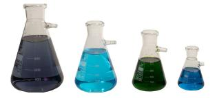
• A filtering flask in engineering testing laboratories is used to hold liquids during filtration processes. It is typically used with a vacuum pump to create suction, which speeds up the filtration of liquids through a filter paper, ensuring the separation of solids from liquids in various chemical or material testing procedures.
