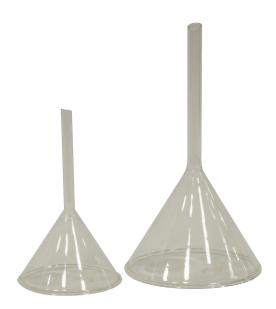
• A glass funnel in engineering testing laboratories is used for transferring liquids or powders into containers with narrow openings. It helps ensure a smooth, controlled flow, preventing spills and contamination, and is commonly used in filtration, sample preparation, and liquid handling processes.
