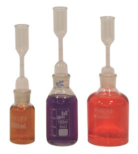
• A pycnometer (bottle type) in engineering testing laboratories is used to determine the density or specific gravity of liquids, powders, or solids. It consists of a sealed glass bottle with precise volume markings, allowing for accurate measurement when filled with the sample and weighed. This method is commonly used for precise measurements in materials testing, especially for liquids and fine powders.
