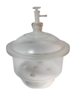
• A vacuum desiccator in engineering testing laboratories is used to store samples in a low-pressure, dry environment. By applying a vacuum, it removes moisture from the air and from the sample itself, ensuring that samples remain dry and uncontaminated during storage or preparation for sensitive tests.
