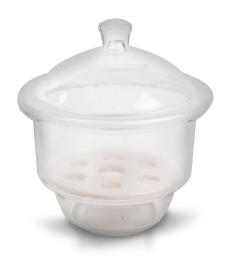
• A desiccator in engineering testing laboratories is used to store samples or materials in a dry environment by absorbing moisture from the air. It helps prevent sample contamination and ensures accurate results in tests that are sensitive to humidity, such as moisture content analysis or when working with hygroscopic materials.
