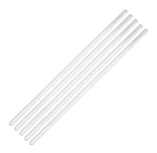
• Stirring bars in engineering testing laboratories are used for mixing liquids or solutions within containers.
