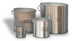
• A unit weight measure in engineering testing laboratories is used to determine the unit weight or density of materials, such as soil or aggregates. It ensures accurate measurement of material properties, which is essential for tests like compaction or specific gravity analysis.
