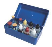
• A water quality test kit in engineering testing laboratories is used to assess various parameters of water, such as pH, turbidity, dissolved oxygen, and chemical contaminants. It helps ensure that water meets environmental and regulatory standards for quality before use in construction or other processes.
