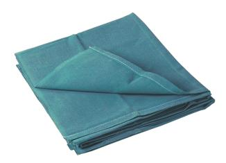
A quartering canvas in engineering testing laboratories is used for reducing bulk soil or aggregate samples to a representative smaller portion by the quartering method. It provides a clean, flat surface to divide and mix materials accurately, ensuring unbiased sampling for testing.
