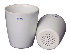
A porcelain crucible in engineering testing laboratories is used for heating, melting, or burning samples at high temperatures. It is chemically resistant and ideal for tasks like determining ash content or performing loss-on-ignition tests without contamination.
