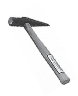
• A density pick in engineering testing laboratories is used to extract and trim soil or asphalt samples to a specific shape and size for density or compaction tests. It ensures accurate specimen preparation, which is essential for reliable test results.
