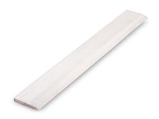
• A straight edge in engineering testing laboratories is used to level and smooth the surface of samples, such as soil in molds, and to check flatness or alignment. It ensures accurate measurements and consistent sample preparation.
