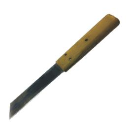
A trimming knife in engineering testing laboratories is used to precisely cut and shape soil or rock samples to required dimensions. It ensures clean, accurate preparation of specimens for testing, improving the reliability of results.
