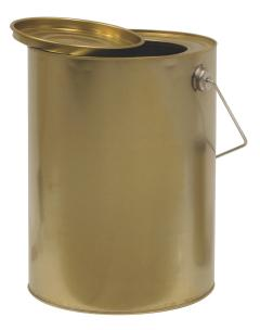
• A sample can in engineering testing laboratories is used to collect, store, and transport material samples such as soil, cement, or aggregates. It protects the sample from contamination and moisture loss, ensuring accurate and reliable test results.
