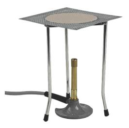
• A Bunsen burner in engineering testing laboratories is used to provide a controlled flame for heating, sterilizing, or combustion tasks. It's essential for experiments requiring open flame and high-temperature conditions, especially in material and chemical testing.
