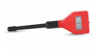
• A pH meter in engineering testing laboratories is used to measure the acidity or alkalinity of materials, especially in soil and water testing. It helps assess chemical properties that affect material behavior, ensuring compliance with standards and supporting accurate analysis for construction and environmental decisions.
