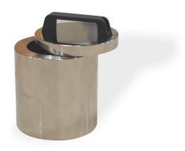
• Used to determine the yield of lime by leaving the specimen to slake in an insulated stainless steel vessel
