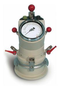
• A cement air meter in engineering testing laboratories is used to measure the air content in fresh cement or concrete mixtures. It helps determine the workability and quality of the mix, ensuring that the correct air-entraining agents are used for achieving desired properties, such as freeze-thaw resistance and improved durability in the final concrete structure.
