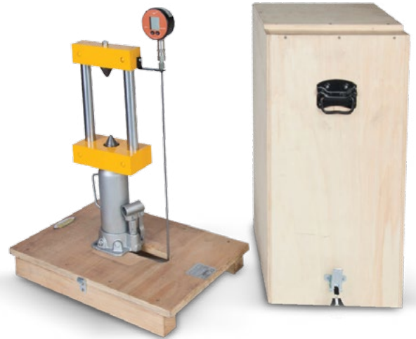
Point Load with Digital Manometer (RM-120)
